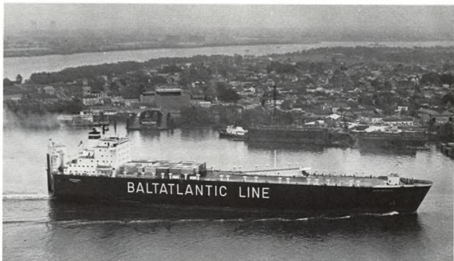
Newest Russian ships carry containers on deck in addition to Ro/Ro cargo. Note ramp to main deck and stern ramp in elevated position as ship visits New Orleans port.
