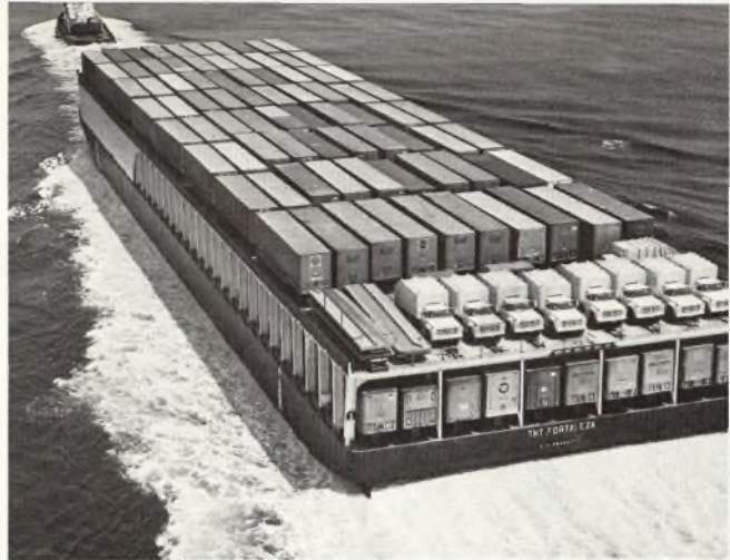
Double-deck Crowley barge, similar to EAST units.
