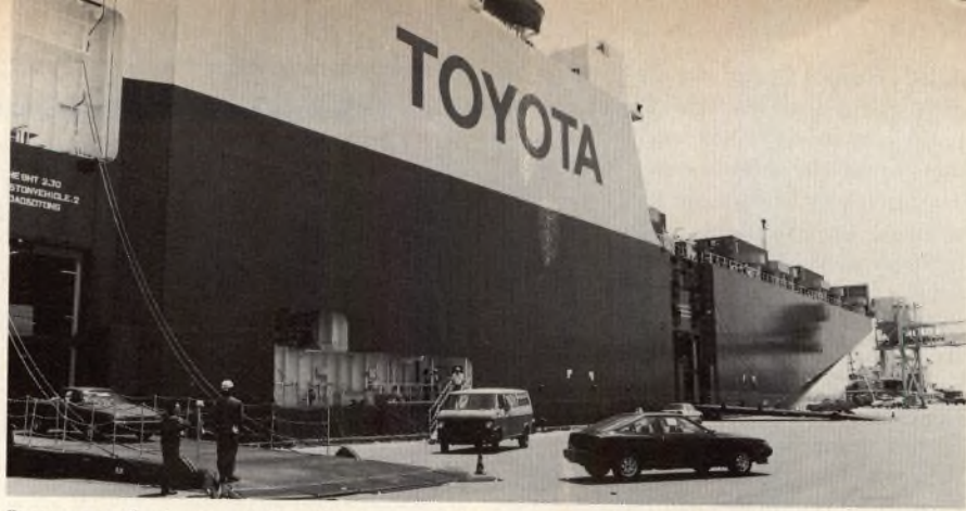
Japan got the jump on Americans by designing ships like the 'M/V Toyo Fuji No. 14' (above) which can carry 4,700 assembled cars plus 120 FEUs of knocked down parts.
