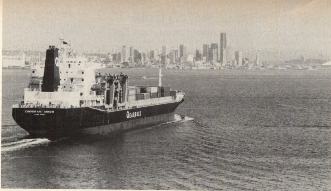
Gearbulk's hybrid 'Cormorant Arrow' is one of 43 sister vessels designed as open-hatch container/forest product carriers.
