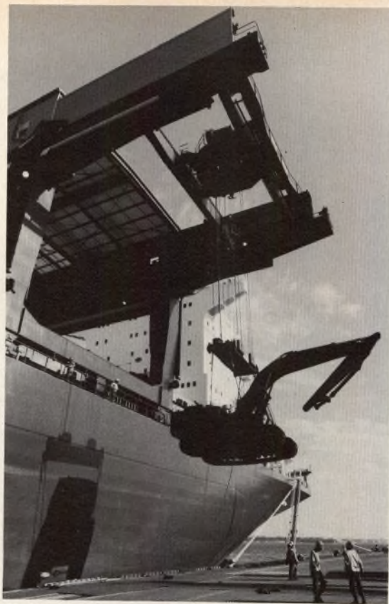
On-board Westwood gantry lifts machinery.
