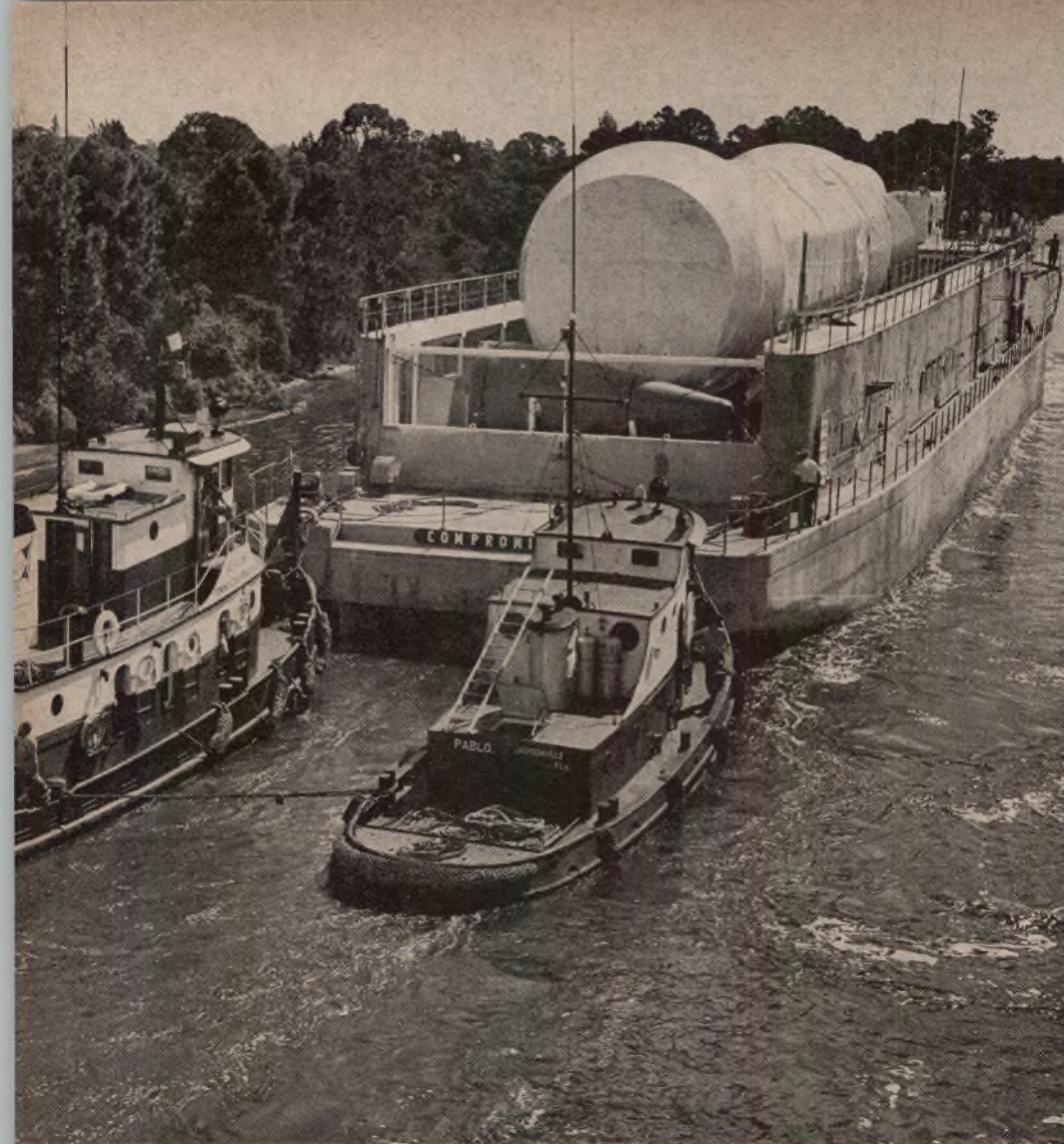
THE SATURN booster barging operation between Huntsville, Ala. and Port Canaveral will not be affected by the new airlift. Above, GATCO barge Compromise is steadily maneuvered through the Intracoastal Waterway to Florida's space center.
